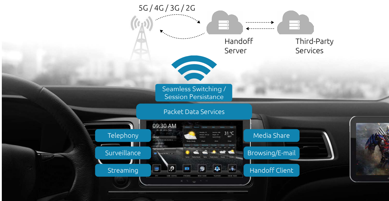
Figure 8: Seamless switching with session persistence based on the edge
